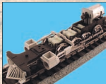
New chassis and drive with four PrimeMover gearboxes, cast-metal drive wheels and rods.
